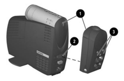
When the adapter is activated, one of the LEDs **3** on the Multimedia Adapter turns green.
